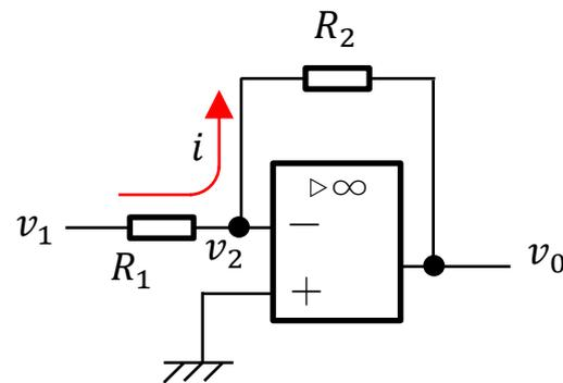
$$v_0 = -\frac{R_2}{R_1} v_1$$
